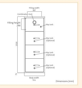
**Chubbsafes Binder Fire File** provides UL 72 Class 350 Endurance certification for up to two hours certified by UL
