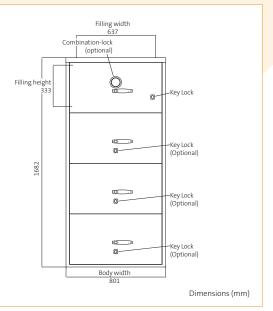
Chubbsafes Lateral Fire File provides UL 72 Class 350 Endurance certification for up to one hour certified by UL.
